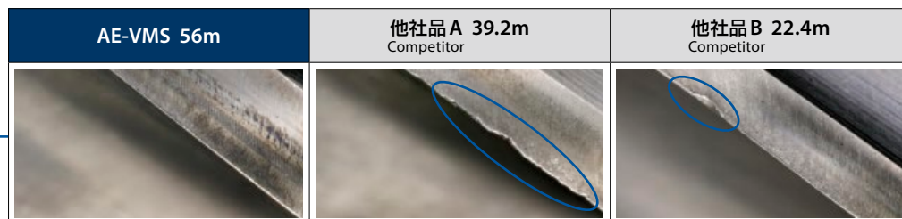
外周刃の損傷状態 Wear comparison of the peripheral cutting edge
