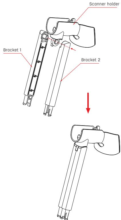
Insert the "screw" into "screw thread" to fix the scanner holder and the brackets.
