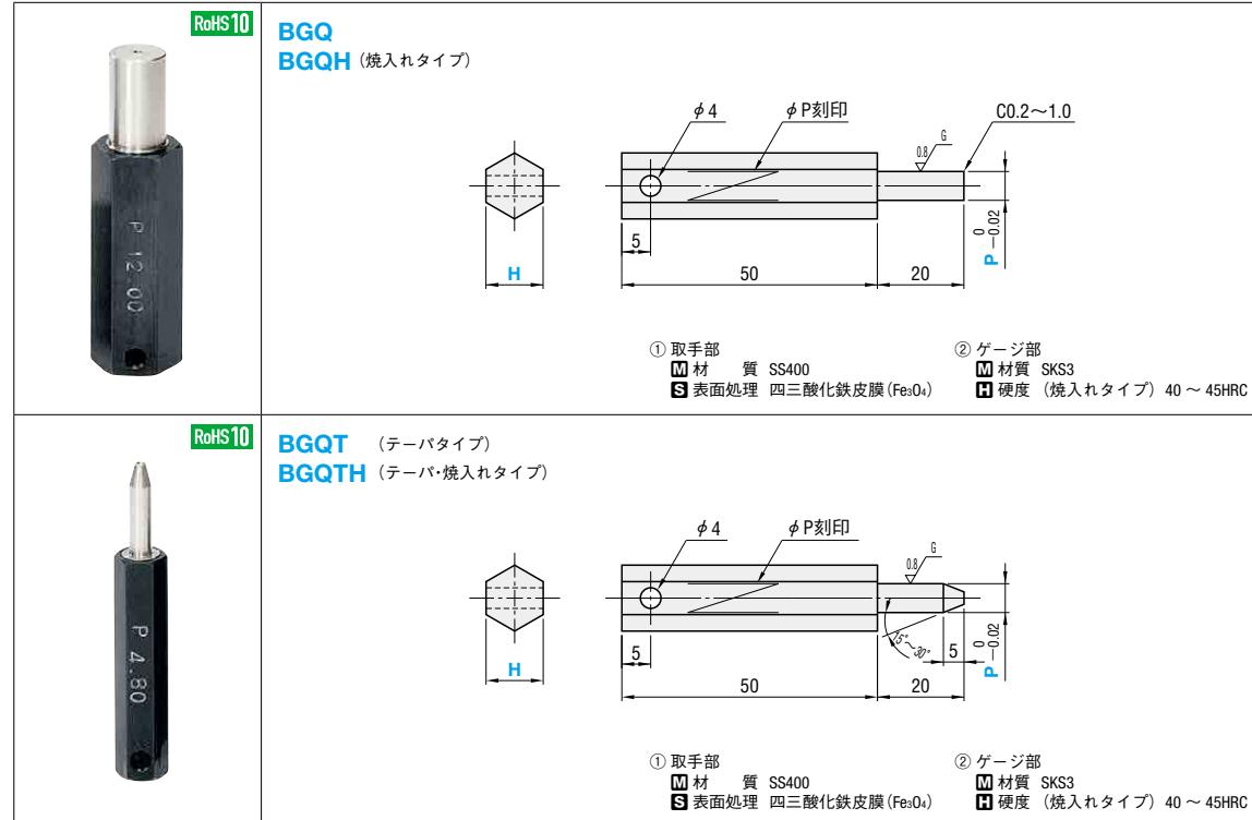
PLUG GAUGES FOR CHECKING FIXTURES - OBLONG TYPE -
