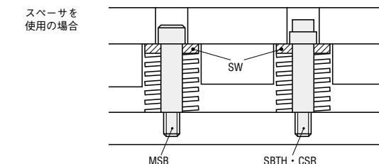
STRIPPER BOLTS, BUSHING TYPE -THICK TYPE-
