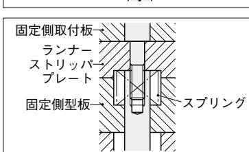
L=固定側取付板厚-(Stop Boltツバ厚K+2)
