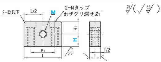
Main specification table for the block with H寸指定タイプ, including columns for H寸指定, M, L, P1, d1, d2, L1, N, and various pitch options.
