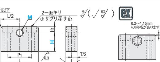
Main specification table for the block with H寸指定タイプ, including columns for H寸指定, M, L, P1, d1, d2, L1, and various pitch options.
