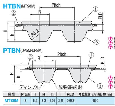
Material and specification tables for HTBN and PTBN belts, including Type, Material (M), and various parameters like Pitch, H, h, L, PLD, and unit weight.
