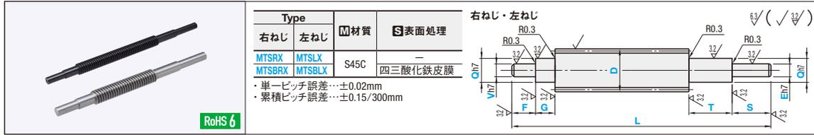
Table with columns: Type, D, L, Q, V・E, Pitch. Lists various screw types and their dimensions.
